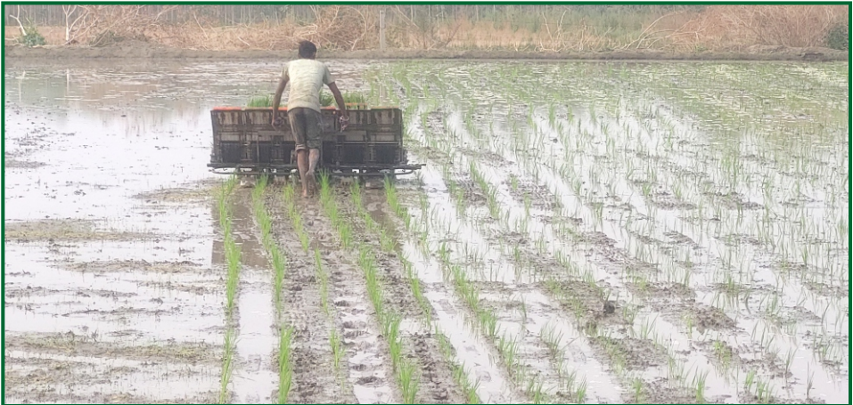
Fig. 2. Self-propelled Walk Behind Paddy Transplanter
